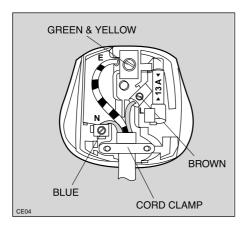
The plug moulded onto the lead incorporates a 13amp BSI362 fuse. Only ASTA or BSI fuses should be used.
