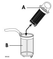
3. Turn the handle about 1/4 a turn anticlockwise and remove.
