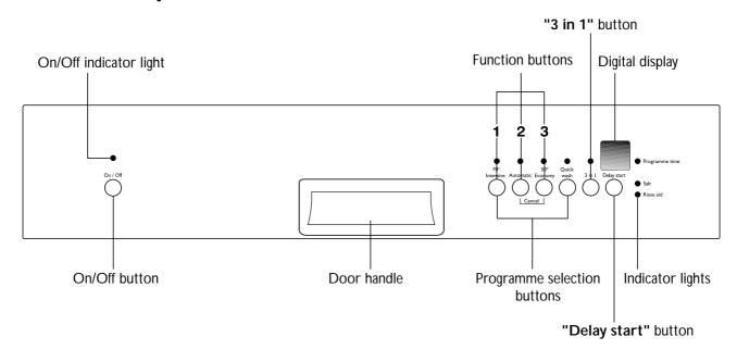
**Function buttons:** in addition to the dishwashing programme selected, the following functions can also be set with the help of these buttons:
