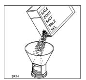
The salt container will require topping up periodically. You are reminded of this by the salt indicator light on the control panel which comes on when the salt has finished.
