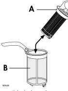
3. Turn the handle about  $^{1\!/_{\!4}}$  a turn anticlockwise and remove.
