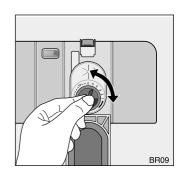
Top up the rinse aid when the indicator light on the control panel illuminates.
