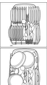
The rows of prongs on the lower basket can be easily lowered to allow you to load pots, pans and bowls.
