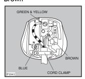
The wire coloured green and yellow must be connected to the terminal marked with the letter «E» or by the earth symbol  $\stackrel{\bot}{=}$  or coloured green and yellow.
