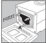
4. Very carefully slide out the right polythene bag, removing it towards the left and then upwards. Remove the bottom cover found inside the drum of your appliance, lay it's hook as the arrow 'A' indicates and push the top of the cover to seal it closed.
