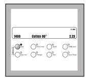
If you press repeatedly the "**Spin**" button it is possible to reduce the spin speed proposed by the machine
