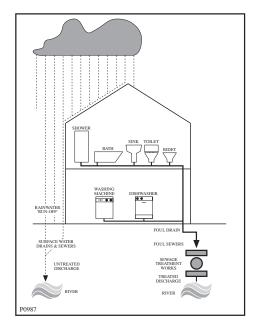
It is essential that these appliances are not connected to the surface water drainage system as this water is discharged directly into a river or stream and may cause pollution.
