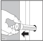
Using a spanner, unscrew and remove the two rear bottom screws. Slide out the two plastic pins. Lay the machine on its back, taking care not to squash the hoses. This can be avoided by placing one of the corner packing pieces between the machine and the floor
