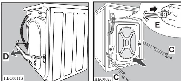
Open the porthole and remove the polystyrene block fitted with the adhesive tape.
