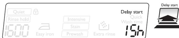
**Before you start the programme**, if you wish to delay the start, press the Delay Start button repeatedly, to select the desired delay.
