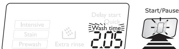
When the calculating phase has finished, the «**Wash time**» stops flashing and the washing time is adjusted to the real load.
