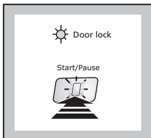
To start the selected programme, press the **Start/Pause** button; the green pilot light stops flashing. If you have selected a delay time, the countdown will begin and will be shown on the display.
