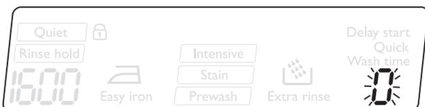
If your laundry is not removed during 10 minutes after the programme has finished, all pilot lights and the display switch off and the energy saving system will be enabled. Only the green Start/Pause light flashes to indicate that the appliance has to be switched off.
