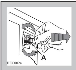
3. Remove the security gasket cup by turning and pulling it away. Pay attention not to move or remove the gasket.
