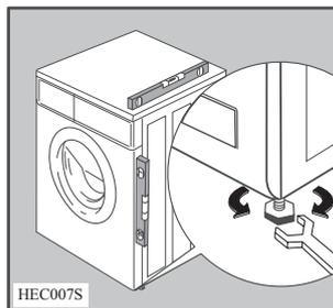
Any necessary adjustment can be made with a spanner. Accurate levelling prevents vibration, (see note on positioning), noise and displacement of the machine during operation.
