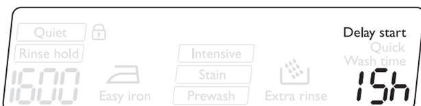
The delay time (20 hours max) is displayed for 3 seconds, then the duration of the selected programme reappears.
